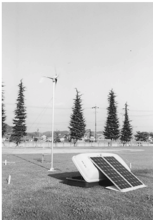
Fig.14 WISH BOX in Operation
