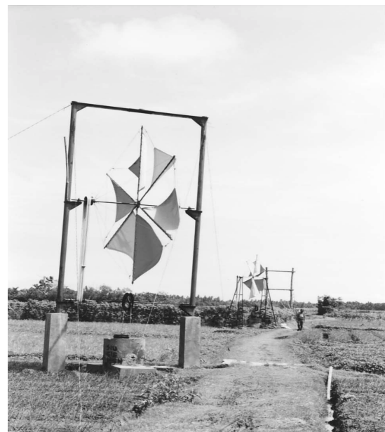
Fig. 2 Cretan type windmill in central Java
